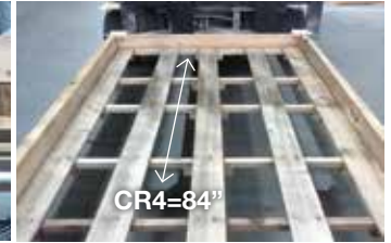
FIG. 5 – CRATE OR A-FRAME – CROSS RUNNERS
